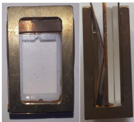
Figure S8: Demountable sandwich cell for fluorescence measurements of hydrated SF:RHD films. Teflon plate of 0.3 mm thickness with a square hole is sandwiched between two quartz plates to prevent evaporation of the hydrated samples. The thin hydrated film was positioned in the gap created by teflon plate. The cell holder is shown in a front (left picture) and side view (right picture).
